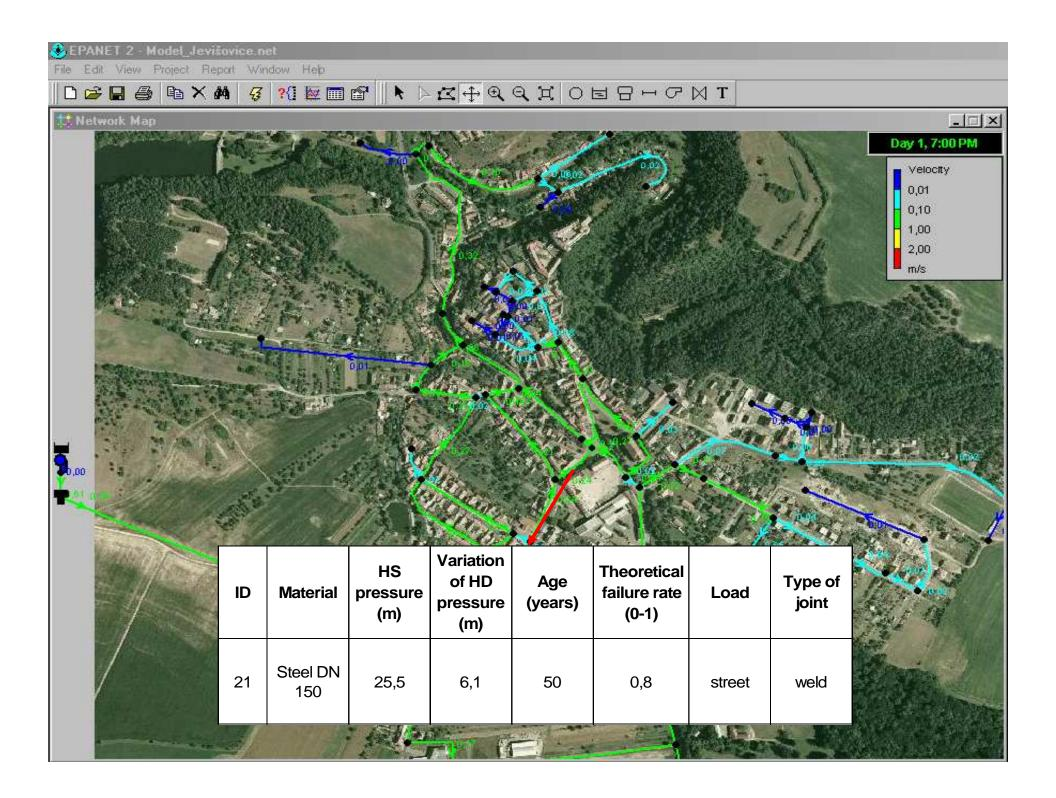
Estimation of **Propability** of pipe failure - driving factors
