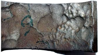
Corrosion is a major reason for bursts and leaks of metallic pipes as well as reduced water quality
